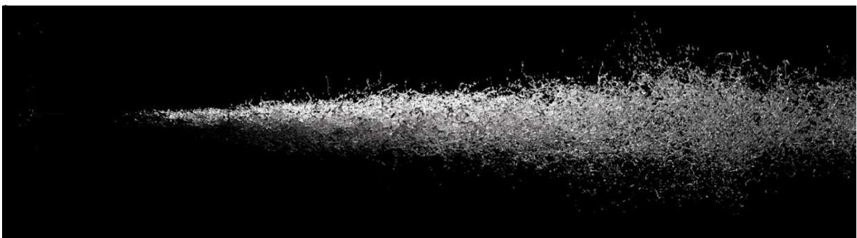
DNS of the primary jet disintegration of a jet consisting of a shear thinning fluid
